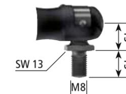
Suitable for ball studs according to DIN 71803 Ø10
