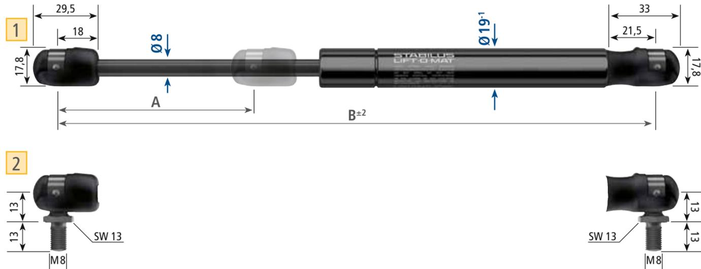
Suitable for ball studs according to DIN 71803 Ø10
