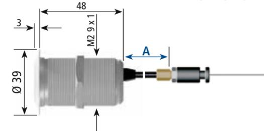
Flush push-button with lateral bowden cable exit
