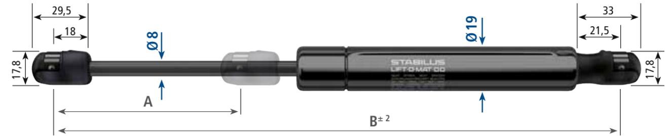
Suitable for ball studs according to DIN 71803 Ø10
