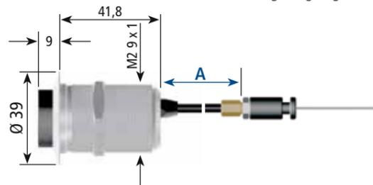
Protruding push-button with lateral bowden cable exit
