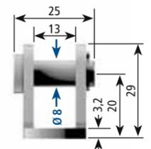
F<sub>max</sub>\* = Maximum allowable force at 20°C in compressed position. Material: steel, zinc-plated.
